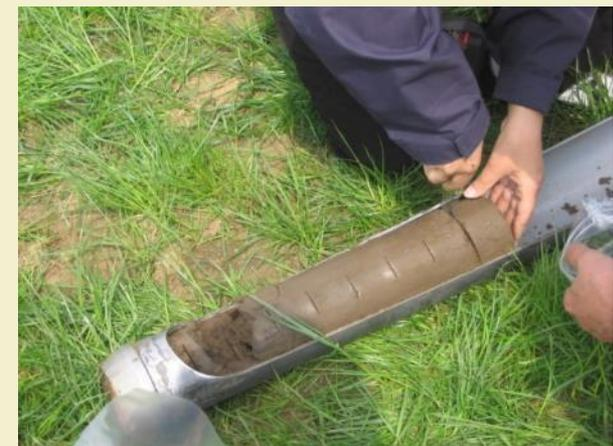
*Incremental depth sampling using the mechanical core sampler*
