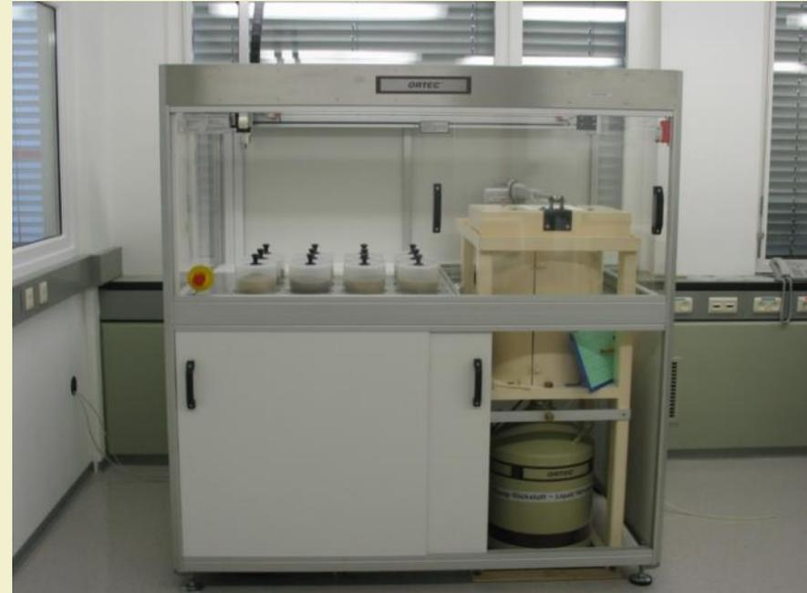
*Fig 2. Gamma spectrometer, Soil Science Unit, IAEA Laboratories, Seibersdorf*
