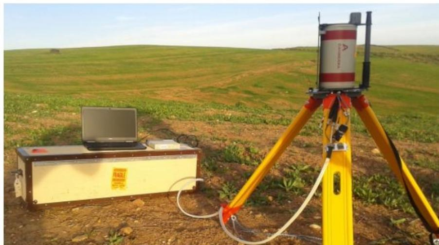
A portable gamma detector provided to the National Centre of Energy, Sciences and Nuclear Techniques in Morocco (CNESTEN). (Photo: CNESTEN)
